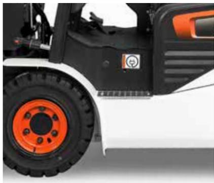
The low anti-slip step and floor plate keep you safe and sound when hopping on and off.
