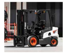
The use of a new U-joint powertrain and oil-cooled disc brakes helps minimize noise and vibration to 77 dBA at the operator's ears.
