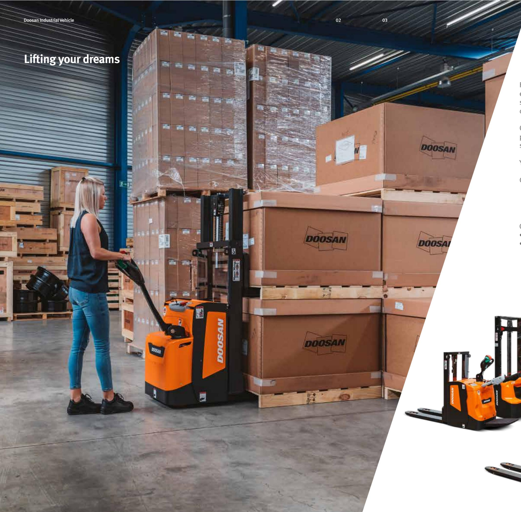
For the various pallet stacking applications that you encounter daily in your warehouse, we offer a durable solution. You can contact us for electric rider stacker and double stackers with a capacity up to 2 tons.
