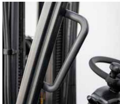
Thanks to the well-placed entry bar and handles, stepping in and out of your vehicle is as quick and comfortable as it gets.
