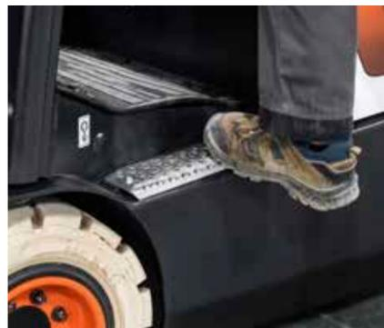
The anti-slip step provides comfortable and safe mounting and dismounting of the vehicle for additional peace of mind.
