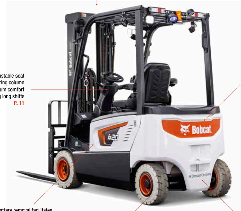
Good visibility through roof enhances operator vision while lifting
